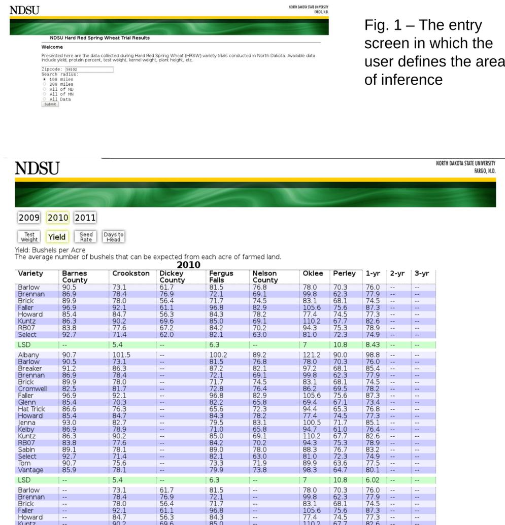
Fig. 2 – Partial WHIP output table for grain yield for all trials within a 100 miles radius of ZIP code 58102 (Fargo, ND), including the single year, across-locations means and LSD ( $\alpha=0.05$ ) values calculated by WHIP.
